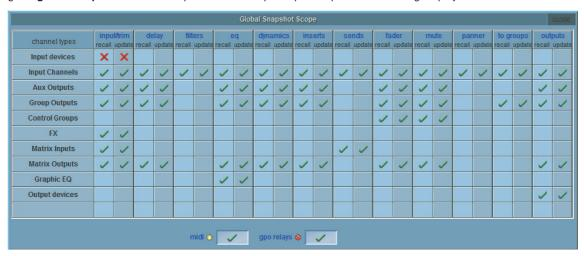
Horizontal rows show the different sections of the console and the vertical rows show the **recall** and **update** status for each of the different types of control. A red X indicates not included, a green tick indicates included, and a blank box indicates that the parameter isn't applicable. These settings can be changed individually by touching the X or tick symbols or by touching the name of a row or column to change all of its contents.
