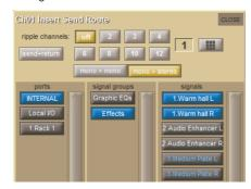
The **send+return** button links the send and return routing for all signals within the **INTERNAL** port: If the **Graphic 1** input is assigned to the insert send, the **Graphic 1** output is automatically assigned to that insert return. Similarly, if it is the return which is manually assigned, the send automatically copies that send assignment. The **send+return** button is grey when inactive and brown when active.
