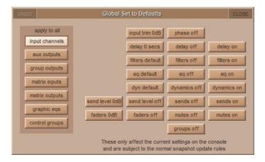
The **Global Set to Defaults** Panel allows global default settings to be applied to the console. Select the Channel type from the list on the left side of the panel, and then select the operation to perform from the available functions.
