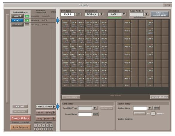
In order to use the rack, the on-screen contents of the rack must match the cards physically installed in the rack connected. There are two ways of achieving this :
