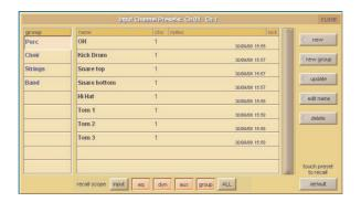
Note that presets are specific to a channel type: The Presets display will only list those presets which apply to the current channel type.
