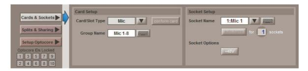
A range of sockets can named with the same label and an incrementing number by using the **auto-name** function below the **Socket Name** box:
