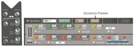
The Assignable encoders and switches beneath the screen can be assigned to any of the main dynamics controls. Hold the Assign Switch button on the left of the input section and touch the dynamics control required on the screen. The selected control is shown by the Status Display.
