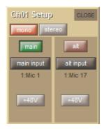
The inputs available on an Input channel include feeds from the external IO racks, the local inputs on the back of the console and a variety of internal signals. Pressing either the **main input** or **alt input** routing button in the **Setup** display opens the **Input Route** display. The signal feeding each input can then be selected as described in the Getting Started section of this manual.
