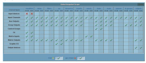
Horizontal rows show the different sections of the console and the vertical rows show the **recall** and **update** status for each of the different types of control. A red X indicates not included, a green tick indicates included, and a blank box indicates that the parameter isn't applicable. These settings can be changed individually by touching the X or tick symbols or by touching the name of a row or column to change all of its contents.
