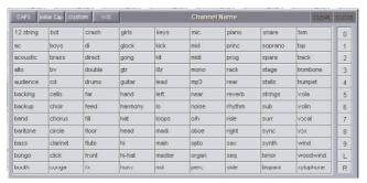
Touching any word from the display inserts that word into the channel name text box. Further words can then be added to the channel name in the same way, divided by a single space. Numeric and L/R identifiers can be added from the column down the right-hand edge of the display. Text can be entered in CAPS or Initial Caps by pressing the CAPS and Initial Cap buttons in the top of the display. If neither of these are selected, all text is inserted in lower case.
