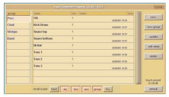
The left-hand column of a preset display contains the available **groups** of presets, and touching one of these groups brings up the list of presets within that group in the column to its right (**name**). The columns to the right of the preset name displays the number of channels whose settings are included in the preset (**chs**) (Channel and Matrix presets only), the date and time it was created or updated (**notes**), and whether or not it is locked (**lock**).
