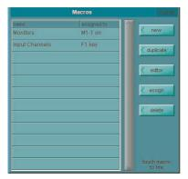
This is where macro commands can be assigned to the **smart keys** in the right-hand section of the console (shown below), as well as to the function (F) buttons on the external keyboard and to the console's GPIs (if implemented). There are four banks of ten smart keys – use the four numbered buttons to their left to switch between banks. Macros can also be fired directly from this list by touching the macro when none of the right-hand buttons is active.
