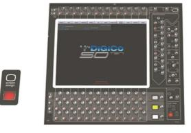
The Left and Right worksurface sections also each have a button labelled **Assign To Centre** which will allow all of the Centre sections controls including faders, mutes and solos to control the bank which has been selected in the Left or Right sections..
