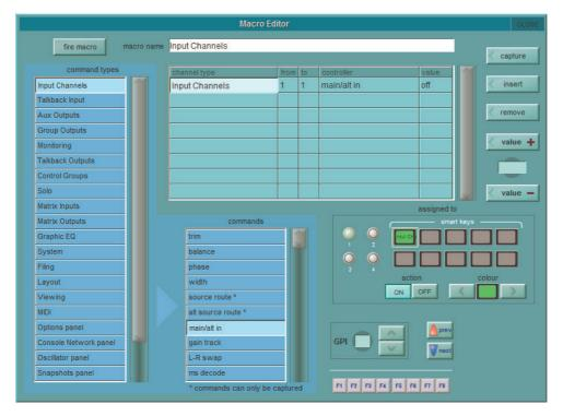
The name of the macro being edited is shown at the top of the display. To switch to a different macro in the list, touch the new macro in the Macro display list (You may need to move the displays around the panel to access the list).
