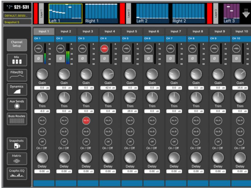
The Channel Setup page will display +48V, polarity, analogue gain, digital trim, channel delay, insert points on/off and meters.
