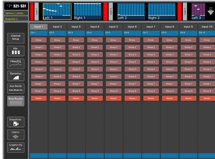
The Buss Routing page allows the assignment of input or group channels to busses. All existing console group busses are represented by buttons and the list can be scrolled vertically by swiping. Channels can also be selected and channel labels edited in this view in the normal way.
