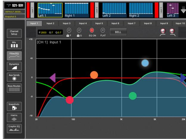
The Filter/EQ page will display the 4 band EQ, HPF/LPF, EQ On/Off and Curve setting
