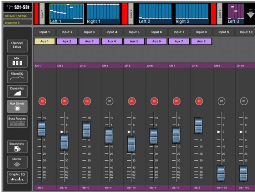
The Aux page will display auxiliary send levels, on/off, auxiliary pans.
