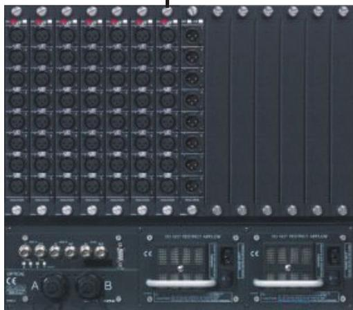
Move Output Card 1 From Slot 8 To Slot 9
