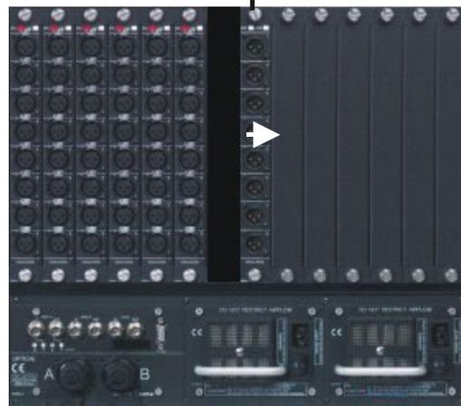
Insert D-Tube in Slot 7 / 8
