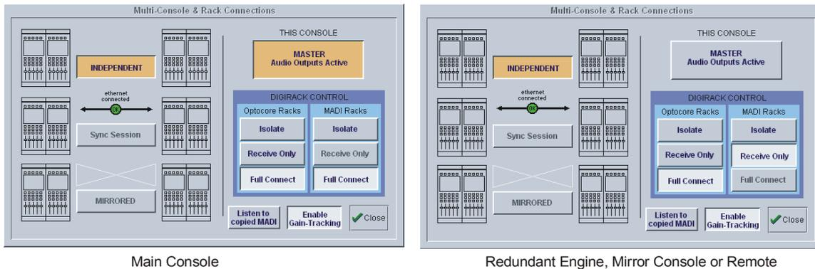
If the system has been defined as consisting of more than one device, the **Consoles & Racks** panel will automatically open on boot up or load session.
