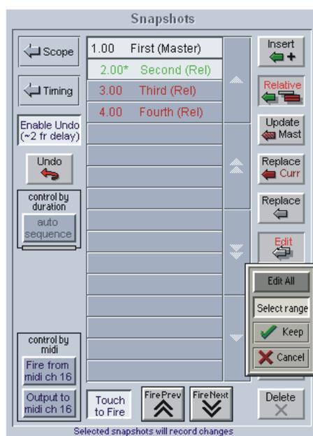
With the Edit button pressed, pressing the Snapshot buttons does not fire the snapshots, it only selects them for editing.
