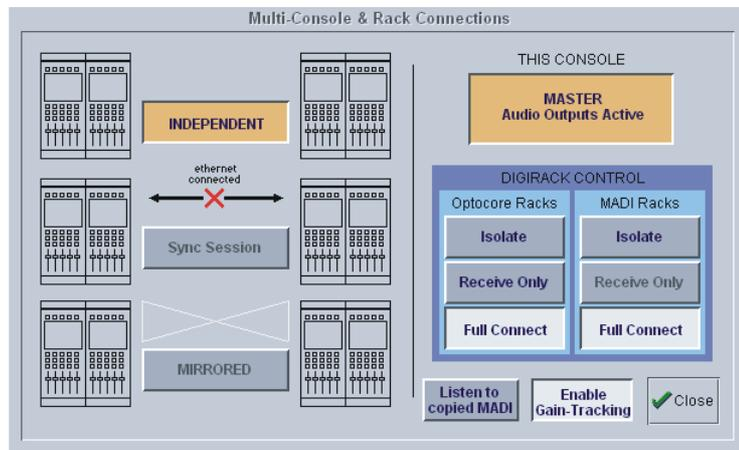
The initial state will have no connection between the devices and the racks (**Isolated**) and the panel appears in order to prompt the operator to make the necessary connections.
