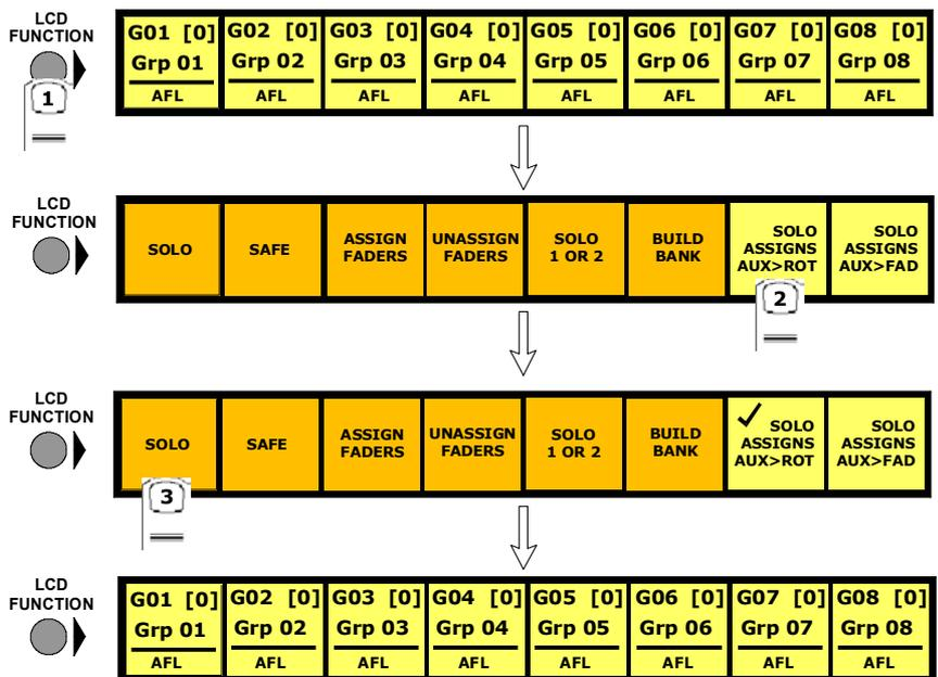
The contents of a Master Fader Bank can be customised at any time by adding or removing faders from it.
