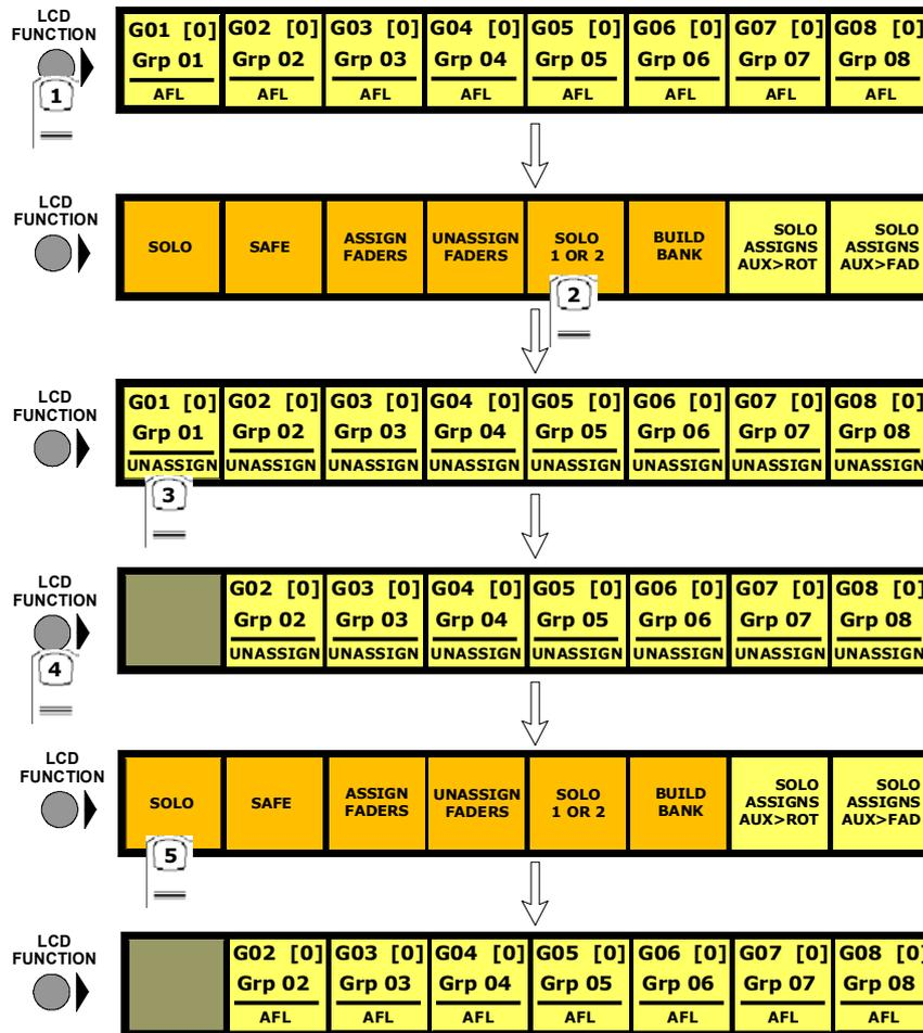
**Master Fader Banks** can also be built from scratch in the following way:
