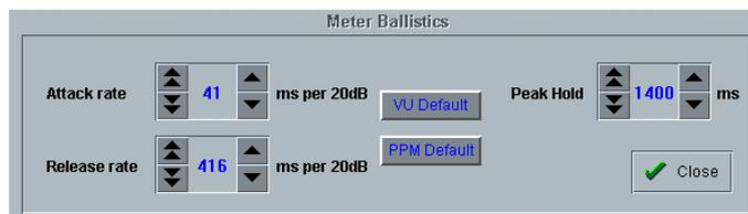
This allows ballistics to be altered for all meters on the bridge and screens using the up/down arrows on the panel.
