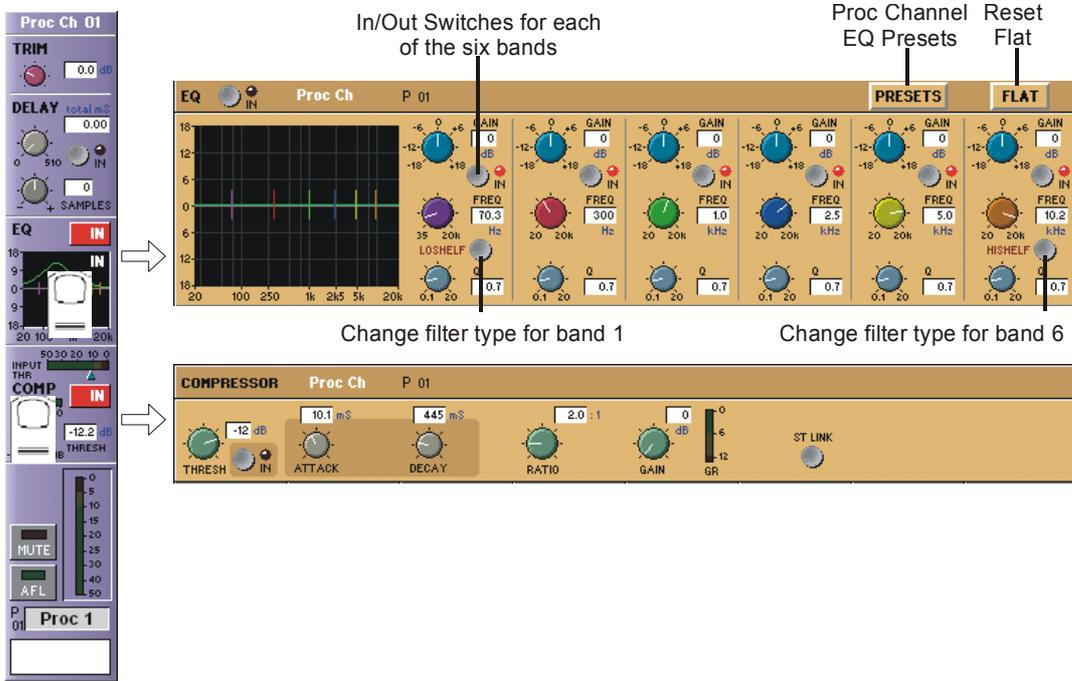
Touching the EQ panel **Presets** button opens the Processing Channel EQ library and this functions in the same way as standard Channel, EQ and Dynamics Presets.
