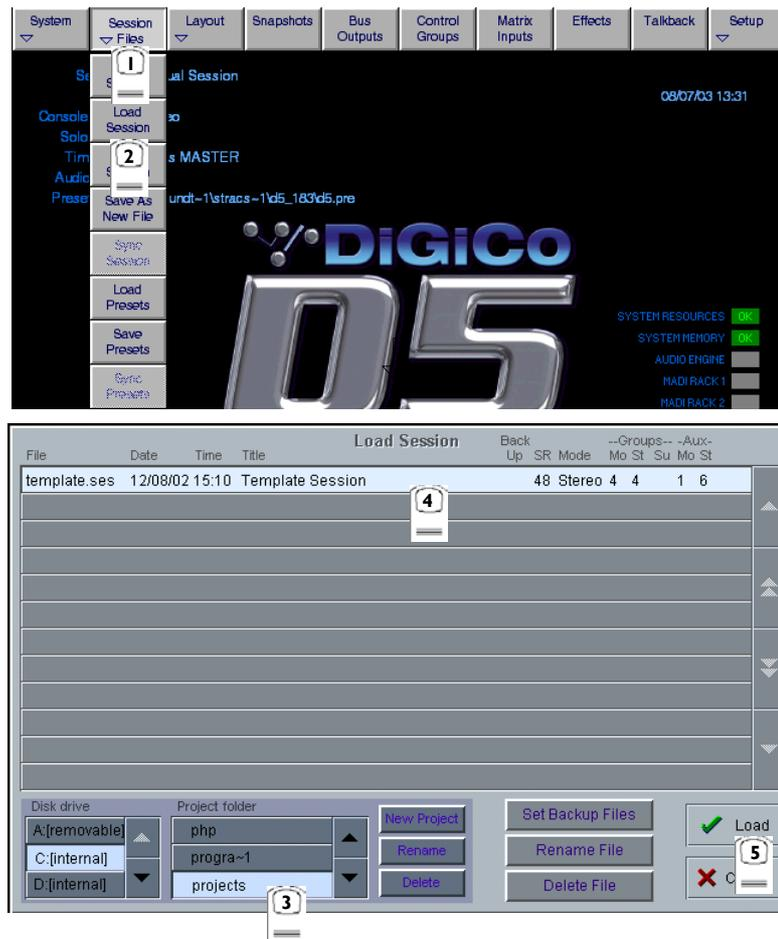
This panel shows the contents of your drives and folders, listing any saved sessions with a note of the console configurations on the right hand side of the screen. These include the removable drive that can be plugged into the USB Data Port on the meter bridge.
