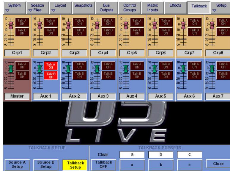
When you first touch the on-screen Talkback button, only the bottom section of the panel is displayed - push the Talkback Setup button to display the full mixer panel.
