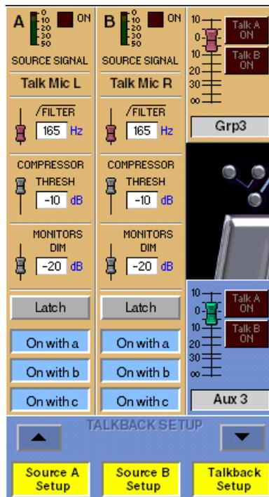
Talkback channels A and B can be sourced from any input signal, the Local (Top) mic, the Rear Mic, Tone or Noise using the buttons at the top of the Channel.
