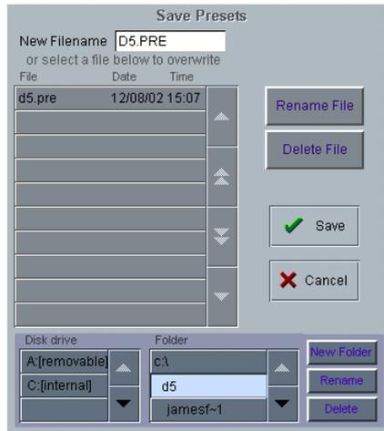
Select a drive and folder in the bottom left hand corner of the panel, type a new name in the **New Filename** box and press the **Save** button.
