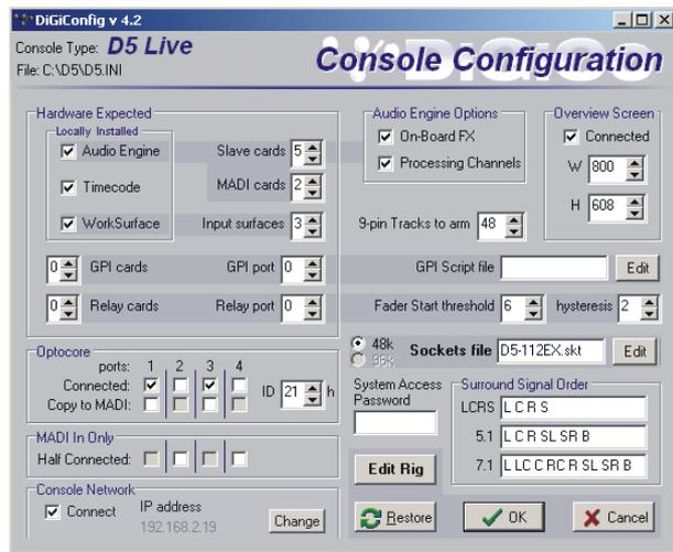
Note that the Optocore IDs are 20 (FOH) and 21 (MIRROR). In this example the network details show that the FOH Main console has an IP address of 192.168.2.11 and the FOH Mirror console has an IP address of 192.168.2.19. All other aspects of the two consoles are identical.
