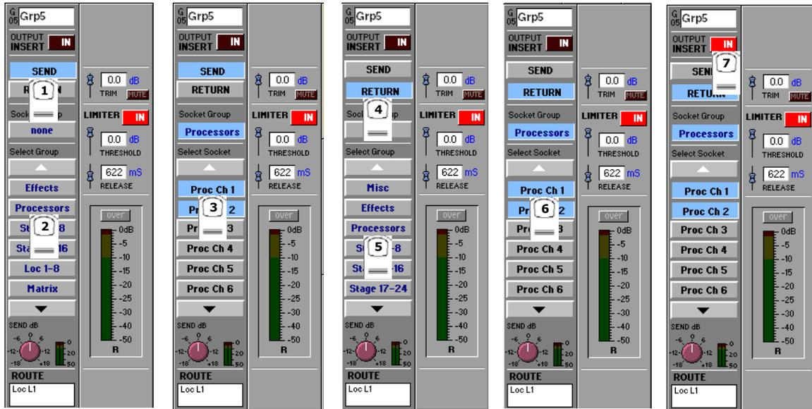
Alternatively, the signal may be sent to the Processing Channel via normal output routing and the Processing Channel can be routed to an output. In the example below, Matrix 1 output is routed to Processing Channel 1 and the processed signal is then routed to Local Line 1.
