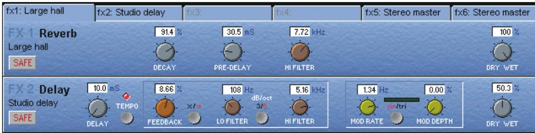
Touch the tabs at the top of the panel to select the effect that you wish to adjust. Normally, two effects modules are shown in the panel but the output processing module uses the whole panel on its own.
