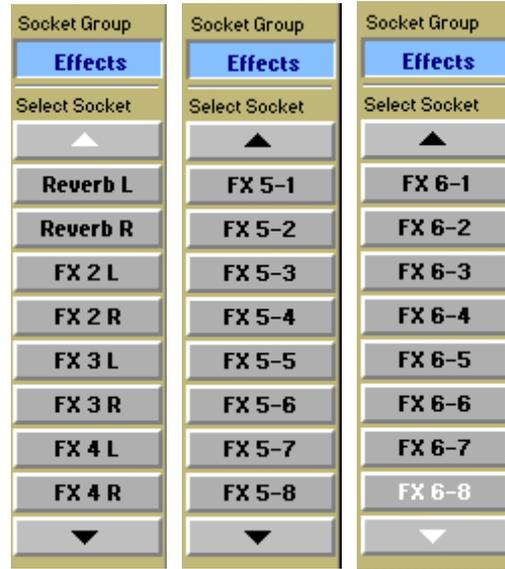
This group contains left and Right sockets for FX 1 to 4 and 8 sockets each for FX5 and FX6. Therefore FX5 and FX6 can be used for output processing on stereo or surround busses.
