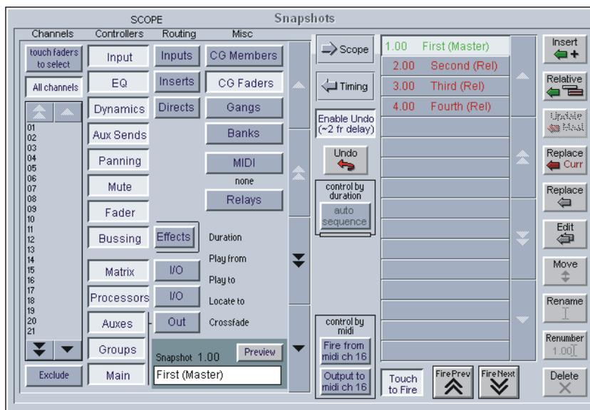
When a snapshot is stored all the console settings are saved but when the snapshot is recalled its effect can be limited to certain channels and controllers.
