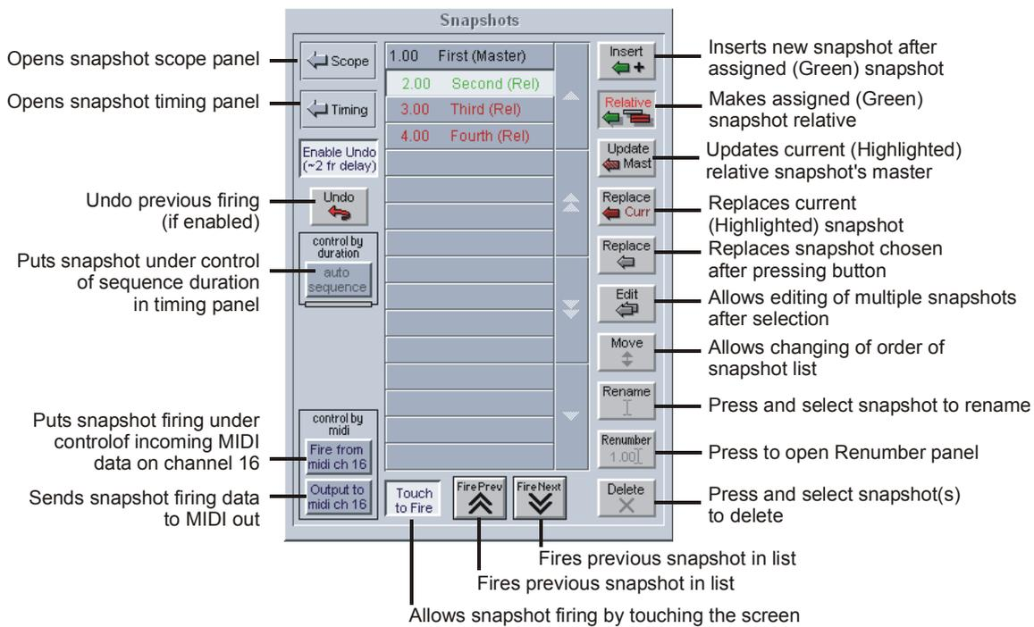
**Note:** The current snapshot appears in the panel as the highlighted (pressed) button. The snapshot name displayed in **green** indicates that it is the assigned to the worksurface and its name is indicated in the display. The **Fire** button recalls this assigned snapshot and highlights it in the screen list as the current snapshot.
