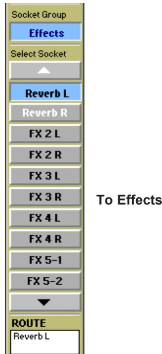
The output of the Reverb module must then be monitored in a channel by opening the input routing screen, selecting the Effects signal group and then selecting Reverb L from the signal list. Touch the **Stereo** button to monitor Reverb L and Reverb R in the same channel.
