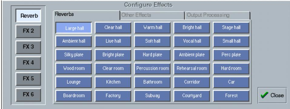
Touch one of the buttons on the left to select an effects module and assign an effect to it by selecting from the grid of buttons labelled with the effect names.
