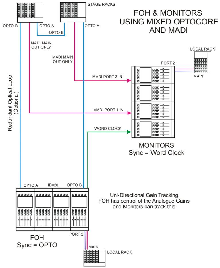
For this setup the **Hardware Configuration** must be manually edited by pressing **Edit Details**.
