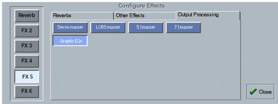
Output Processing consists of input and output gain, 3 band compression and limiting and 4 band EQ for each channel.
