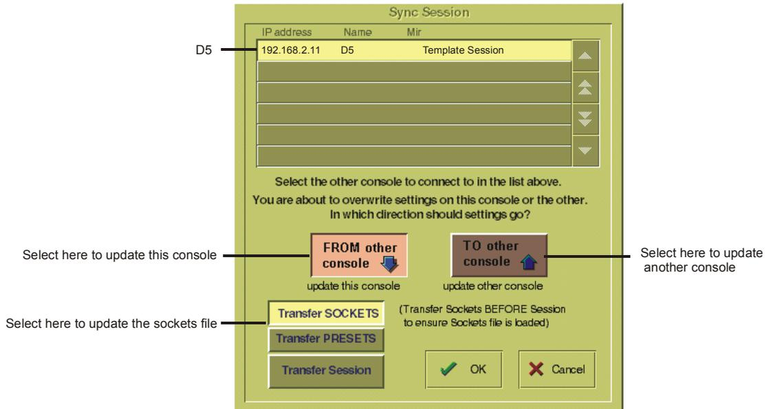
This shows a list of the devices that are connected on the network and in this example there is a D5.
